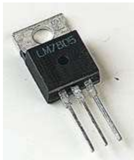
Fig .A Three Terminal Voltage Regulator
